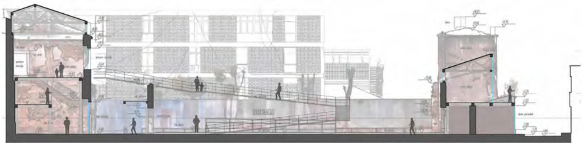
Figure 9: Longitudinal section showing the relation between the historic buildings, the ramp, and the courtyard
