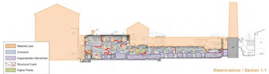
Figure 2: Unkapanı Flour Mill deteriorations in elevation (Modified from Alper, 2021)
